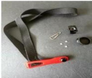
**Gambar 1.** TLD *chip*, *holder* 'eye-D' TLD lensa mata, dan *holder* TLD cincin [1]
